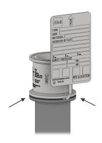
**5.** Assemble unit with sanitary clamp. Both ferrules must fit inside clamp groove prior to tightening the clamp.
