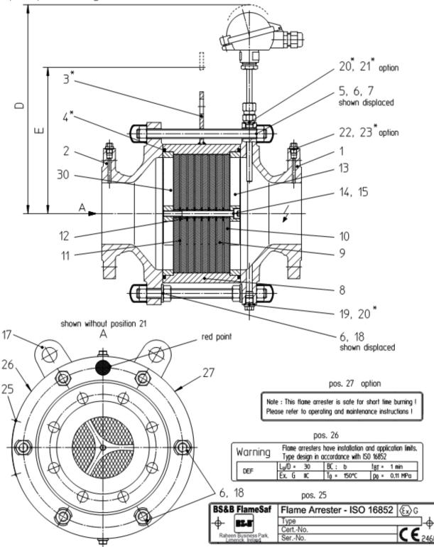
Note: Parts marked with \* shall be available for maintenance works... Dimension D and E are dismantling dimensions.
