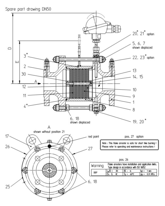
Note: Parts marked with \* shall be available for maintenance works... Dimension D and E are dismantling dimensions.
