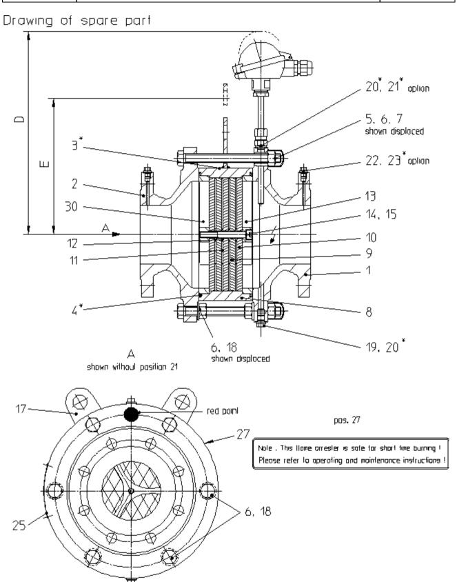
Attention: Parts marked with \* shall be available for maintenance works.
