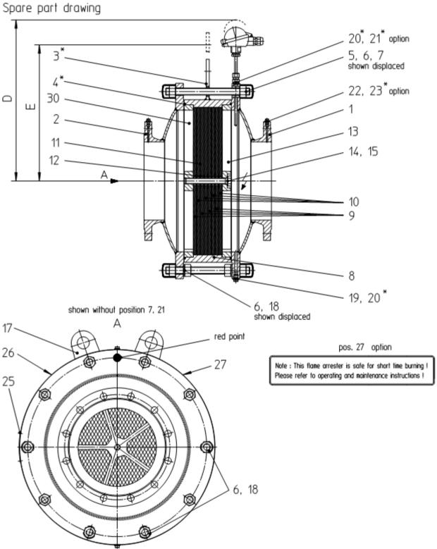
Note: Parts marked with \* shall be available for maintenance works. Dimensions D and E are dismantling dimensions.
