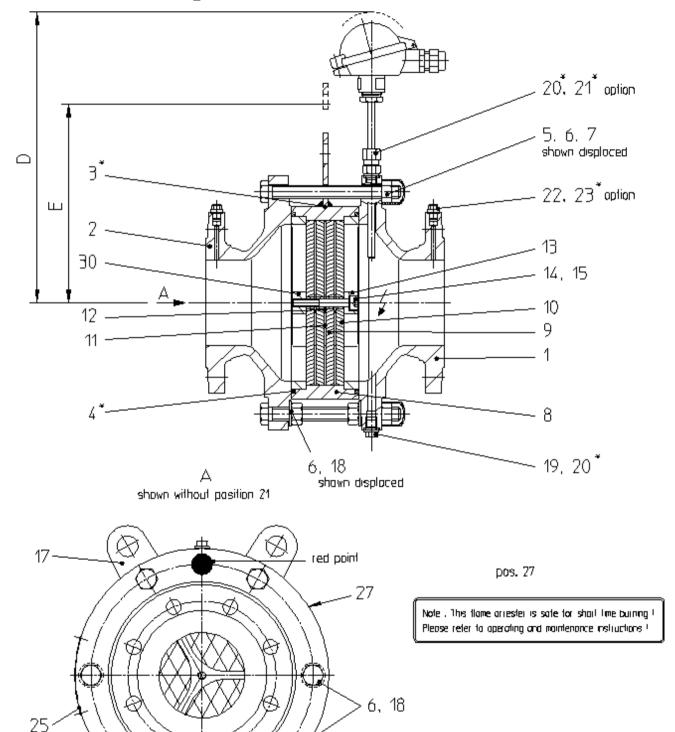
Attention: Ports marked with  $\star$  shall be available for maintenance works. Dimension D and E are dismantling dimensions.
