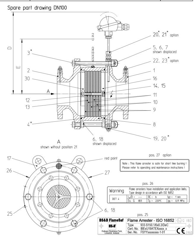
Note: Parts marked with  $\star$  shall be available for maintenance works. Dimension D and E are dismantling dimensions.
