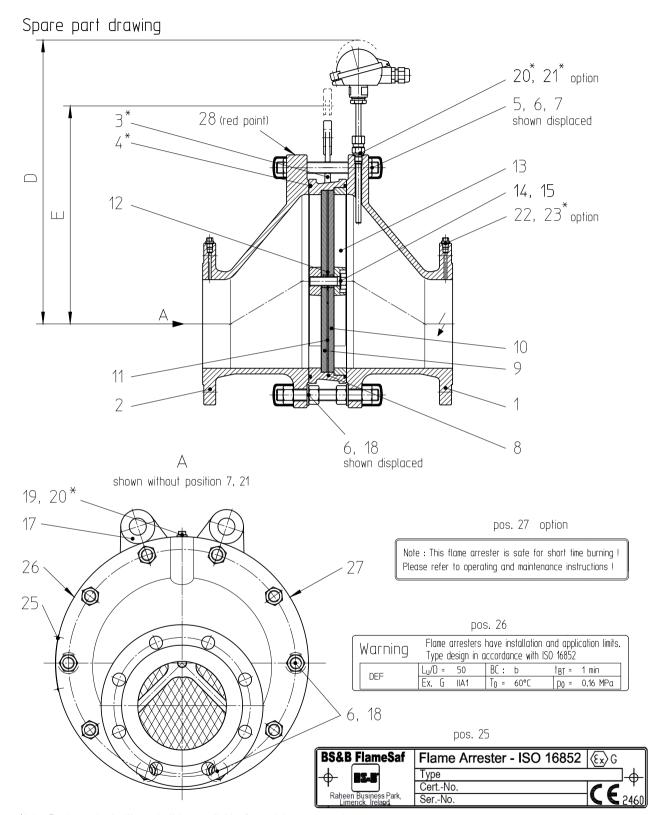
Note: Parts marked with  $\star$  shall be available for maintenance works. Dimensions D and E are dismantling dimensions.
