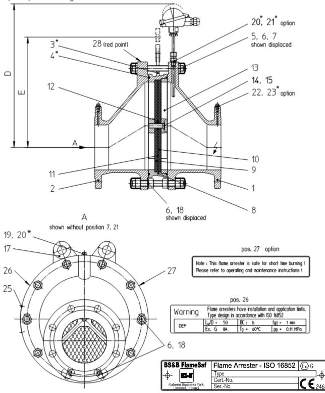
Note: Parts marked with \* shall be available for maintenance works. Dimensions D and E are dismantling dimensions.
