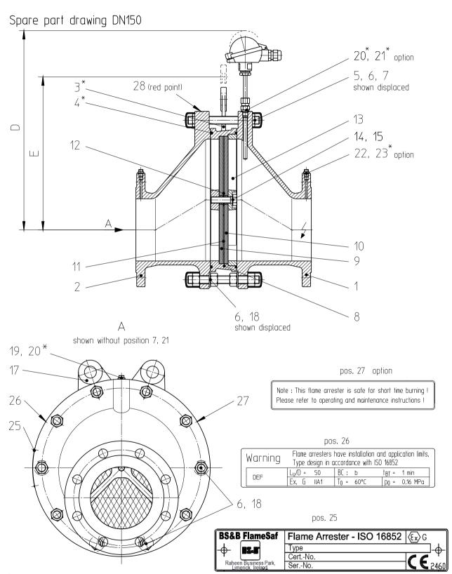
Note: Parts marked with \* shall be available for maintenance works.
