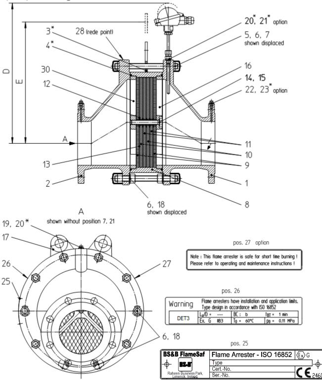
Note: Parts marked with \* shall be available for maintenance works. Dimensions D and E are dismantling dimensions.
