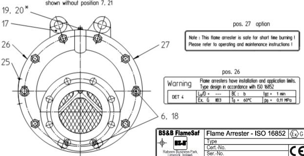
Note: Parts marked with \* shall be available for maintenance works. Dimensions D and E are dismantling dimensions.
