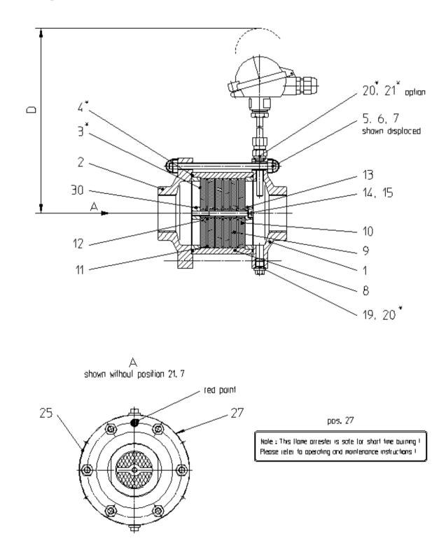
Attention : Parts marked with \* shall be available for maintenance works. Dimension D is a size in dismanified condition.
