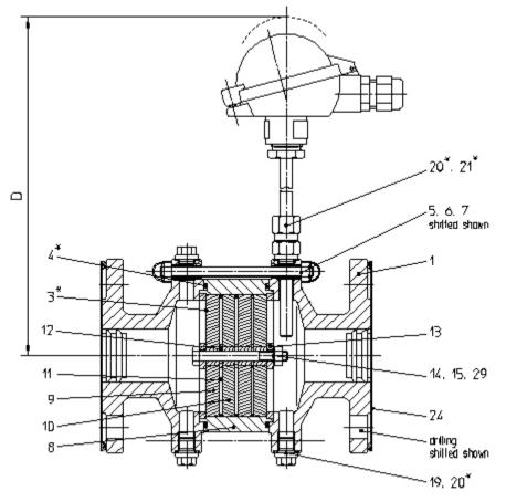
Attention: Parts marked with \* shall be available for maintenance works. Dimension D is a dismantling dimension.
