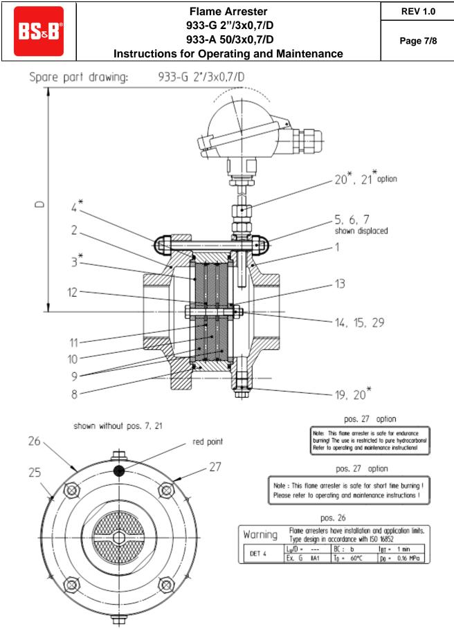
Note: Parts marked with \* shall be available for maintenance works. Dimension D is a size in dismantled condition.
