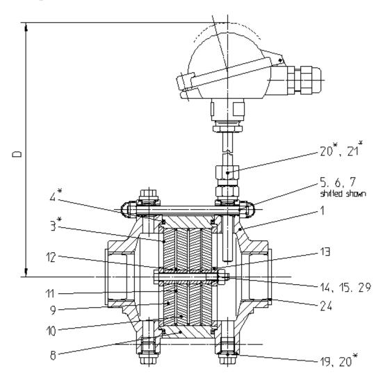
Attention . Parts marked with \* shall be available for maintenance works. Dimension D is a size dismaniled condition.
