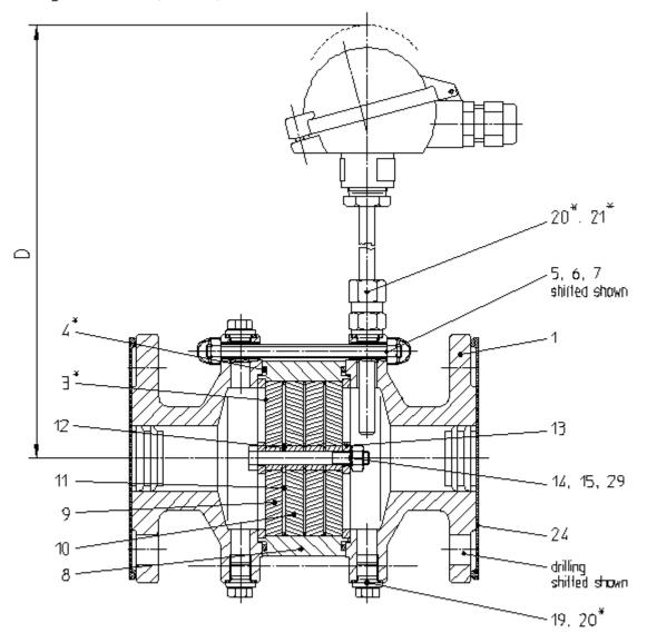
Attention : Parts marked with  $\times$  shall be available for maintenance works. Dimension D is a size dismontled condition.
