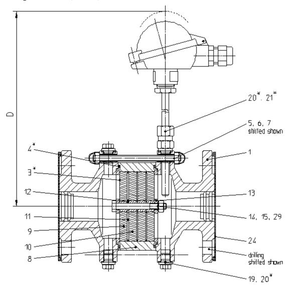
Attention : Parts marked with  $\times$  shall be available for maintenance works. Dimension D is a size dismantled condition.
