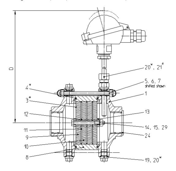
Attention . Parts marked with  $\star$  shall be available for maintenance works. Dimension D is a size dismanlled condition.
