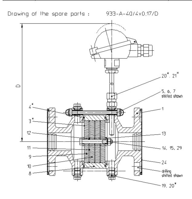
Attention : Parts marked with  $\times$  shall be available for maintenance works. Dimension D is a size dismontted condition.
