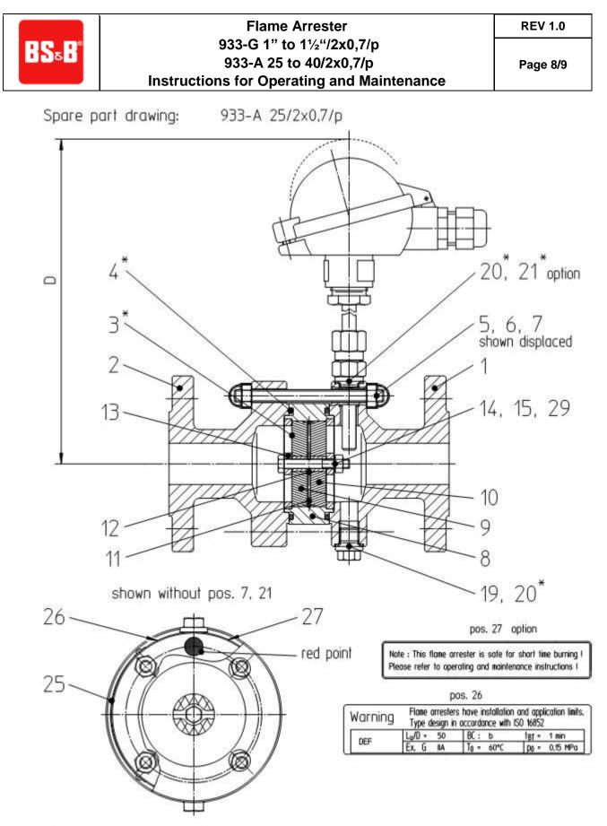
Note: Parts marked with \* shall be available for maintenance works. Dimension D is a size in dismantled condition.
