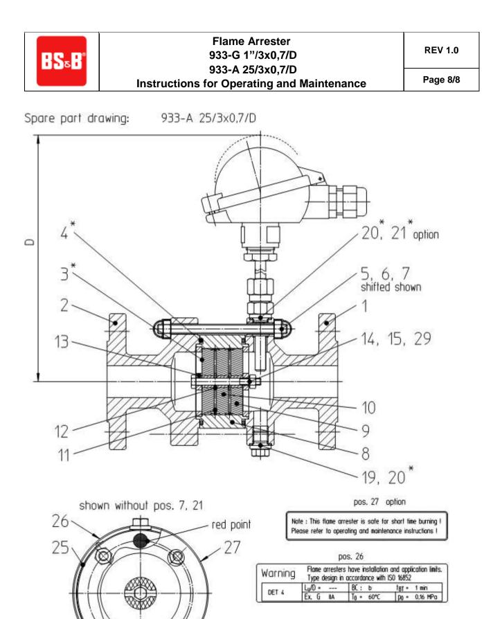
Note: Parts marked with \* shall be available for maintenance works. Dimension D is a size in dismantled condition.
